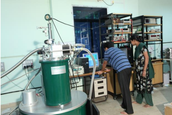
Cryogen free 10T superconducting magnet with 2K variable temperature inserts
