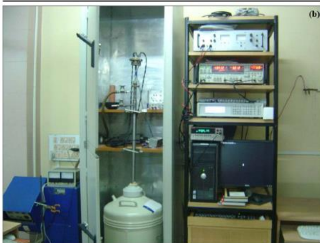
Home made set-up to measure the 1/f Noise and Nyquist noise. The set-up is kept in a shielded enclosure
